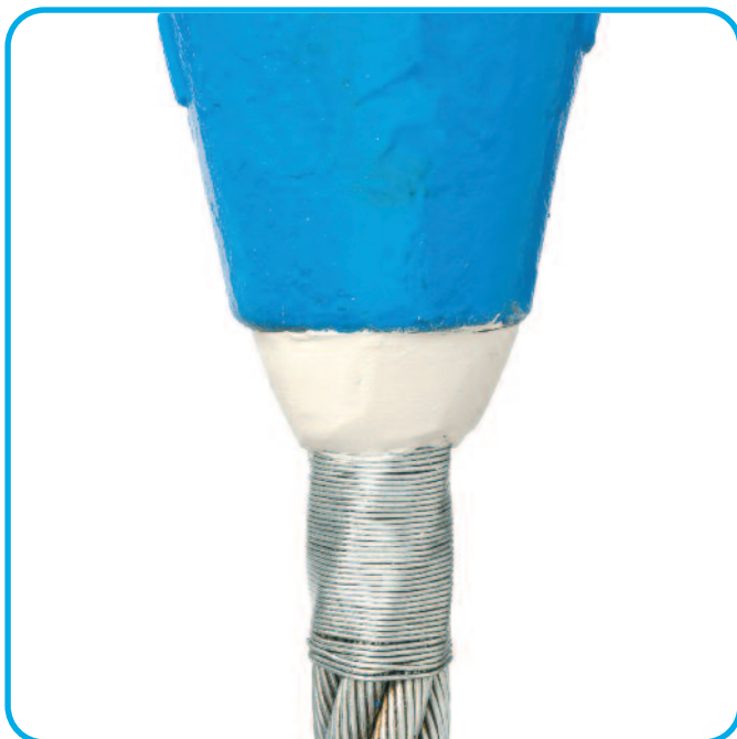
Figure 7: Axes of socket and rope properly aligned and sealed with WIRELOCK® putty/ clay.
