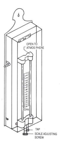
Improved 'NMC' Water Gauge comprise two no 6mm straight corning glass tubes terminating into a brass block with a connecting passage. One limb is open to atmosphere & other is connected to fan drift. A tap is provided to close the connection while taking reading. A scale with adjusting screw is mounted behind the glass tubes. A spirit level helps in keeping the instrument vertical.
