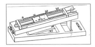
a) At right angle for measurement of large pressure difference.
